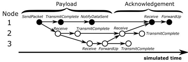
Figure 7: Event patterns in the TCP/IP model: a single packet is transmitted from node 1 to 3 via node 2. Node 3 replies with an acknowledgement.
