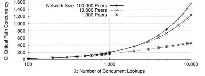
Figure 4: Results of sensitivity analysis of the Kademlia model with  $\alpha = 8$ , varying the number  $\lambda$  of concurrent lookups.
