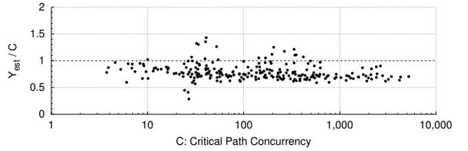
Figure 16: Comparison of our analytical estimate ( $Y_{est}$ ) with critical path concurrency ( $C$ ) of the Kademia model.
