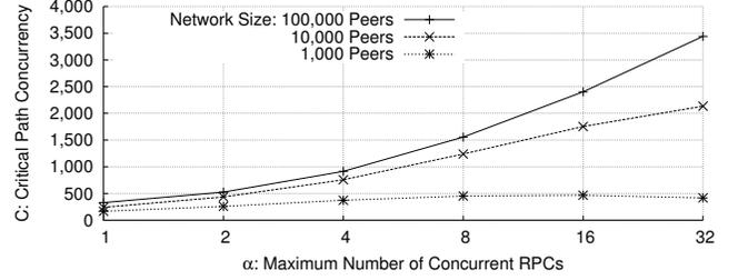
Figure 5: Results of sensitivity analysis of the Kademlia model with  $\lambda = 10,000$ , varying the number  $\alpha$  of concurrent RPCs per lookup.
